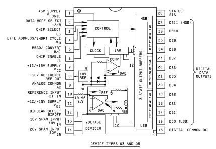
FIGURE 3. Block diagram.
