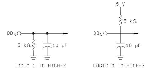
FIGURE 7. Load circuit for output float delay test.
