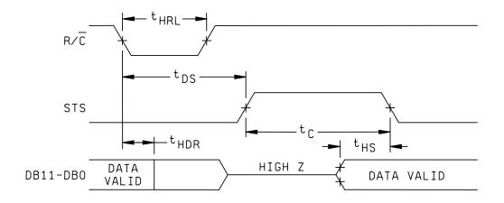
LOW PULSE FOR R /  $\overline{\mathsf{C}}$  - OUTPUTS ENABLED AFTER CONVERSION
