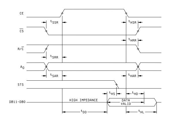
FIGURE 6. Read cycle timing.
