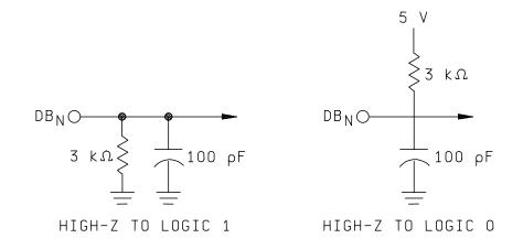
FIGURE 8. Load circuit for access time test.
